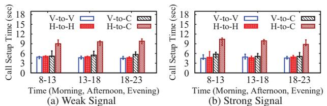
**Figure 2: Call setup time (maximum, median, minimum) in weak-signal(a) and strong-signal(b) scenarios.**
